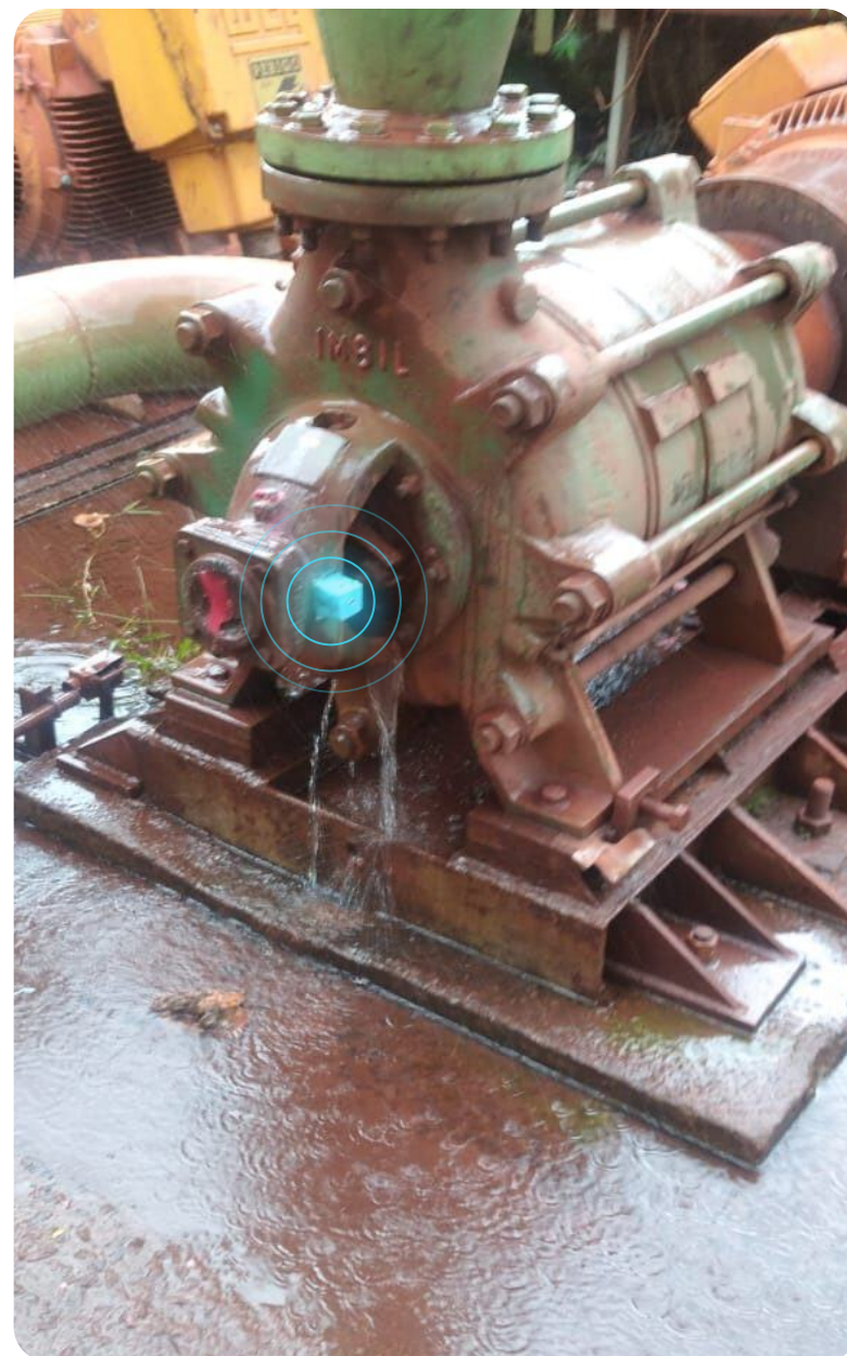
Gasket temperature monitoring to indicate leaks.
