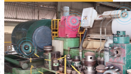
Positive displacement pumps, internal monitoring inside the bearing housing.
